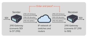
In the diagram above, the cloud represents a network of switches and routers, and the 2110 gateways provide conversion from SDI to ST 2110 to pass through the IP network, and then conversion from ST 2110 back to SDI at the receiving side. All these elements require testing.
