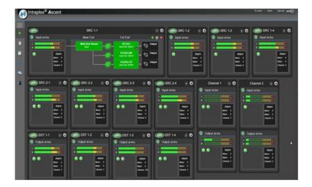
Built on the proven, award-winning Intraplex® IP Link codec technology, GatesAir's Intraplex Ascent platform supports up to 32 audio channels with high-end features.
