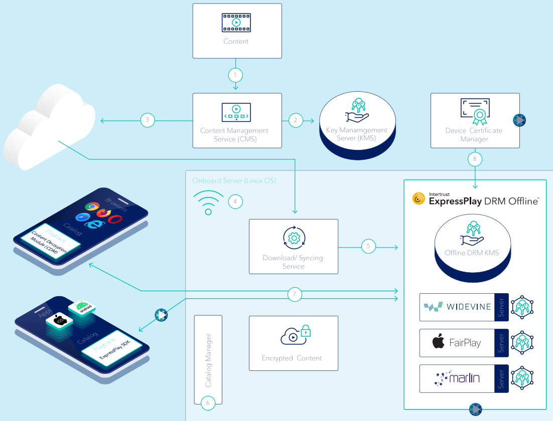
Fig. 1 The secure offline streaming architecture with key components and secure workflow
