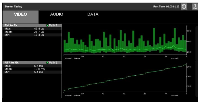
ST2110-20 timing against PTP and packet latency trend graph
